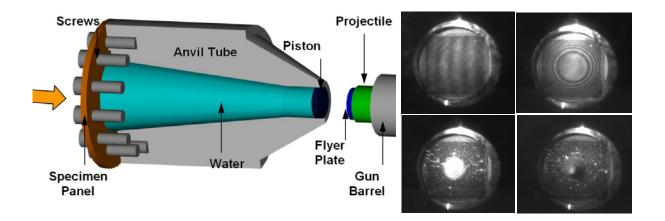
a) Configuration of Fluid-Structure Interaction (FSI) experimental setup. b) Sequence of highspeed images obtained by Shadow Moiré.
